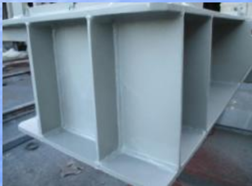
Application status of undercoat material
