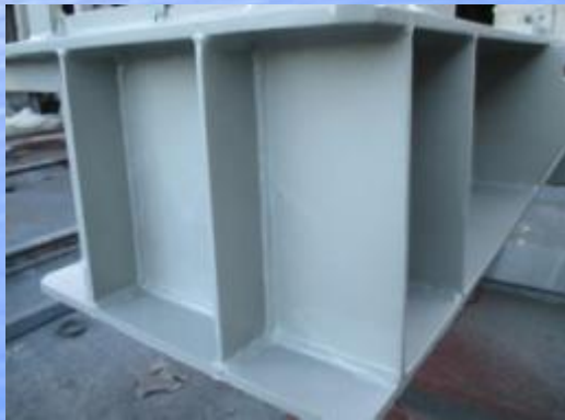
Application status of undercoat material
